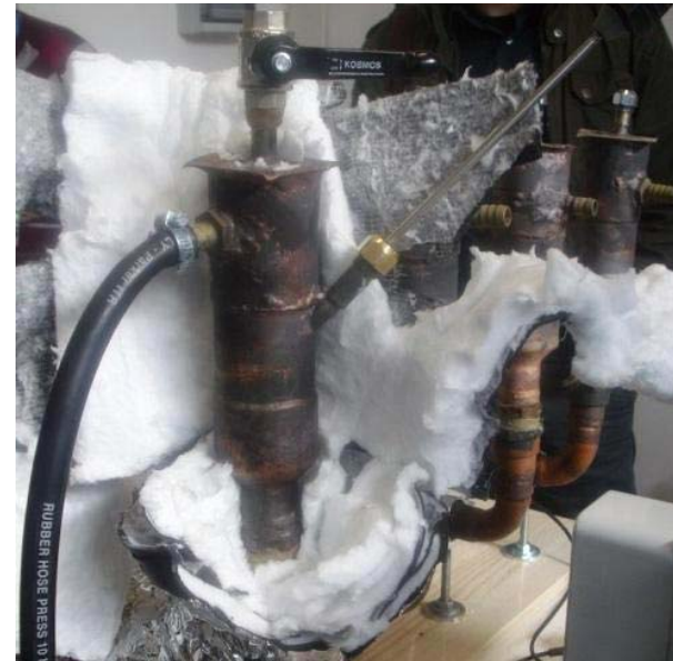
Figure showing the chimney with the black outlet tubing, the thermocouple holder and on the top, the steam exhaust valve.
